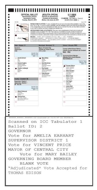
mark. The pixel count of each mark is compared with two thresholds (which are customer configurable. to determine what constitutes a vote.
